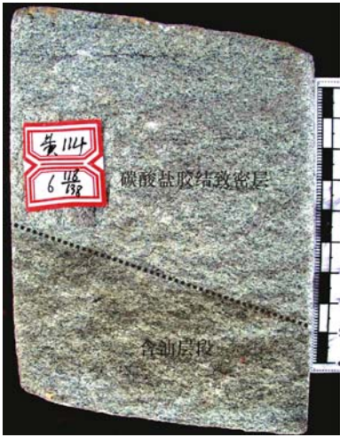
图 5 红井子地区钙质夹层对石油的遮挡作用 Fig. 5 Sealing effects of calcareous interlayers on hydrocarbon accumulation in Hongjingzi area
